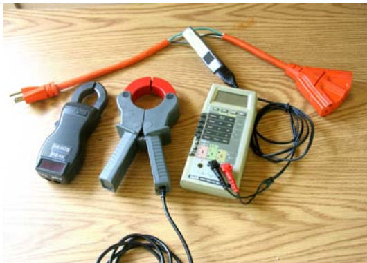
Fig 20 – Current probes and breakout cable
